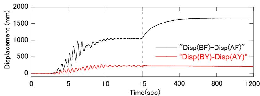
Figure 3. Relative horizontal displacements of quay-walls and footings in A-side and B-side (Case 2)
