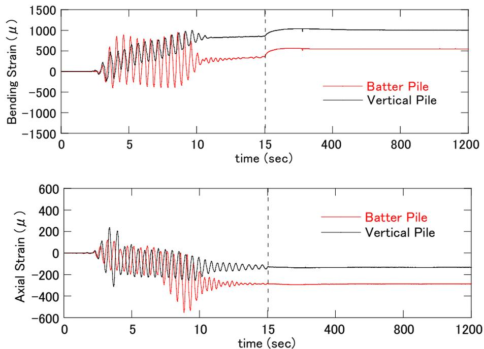
Figure 8. Comparisons between the time histories of the axial and bending strains of the vertical and batter piles at the pile-head: BS1 (Case 32)
