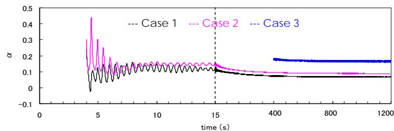
Figure 4. Influence factor  $\alpha$  of Case 1 to 3. Effect on the horizontal displacement of the footing to unit horizontal displacement of the collapsed quay-wall
