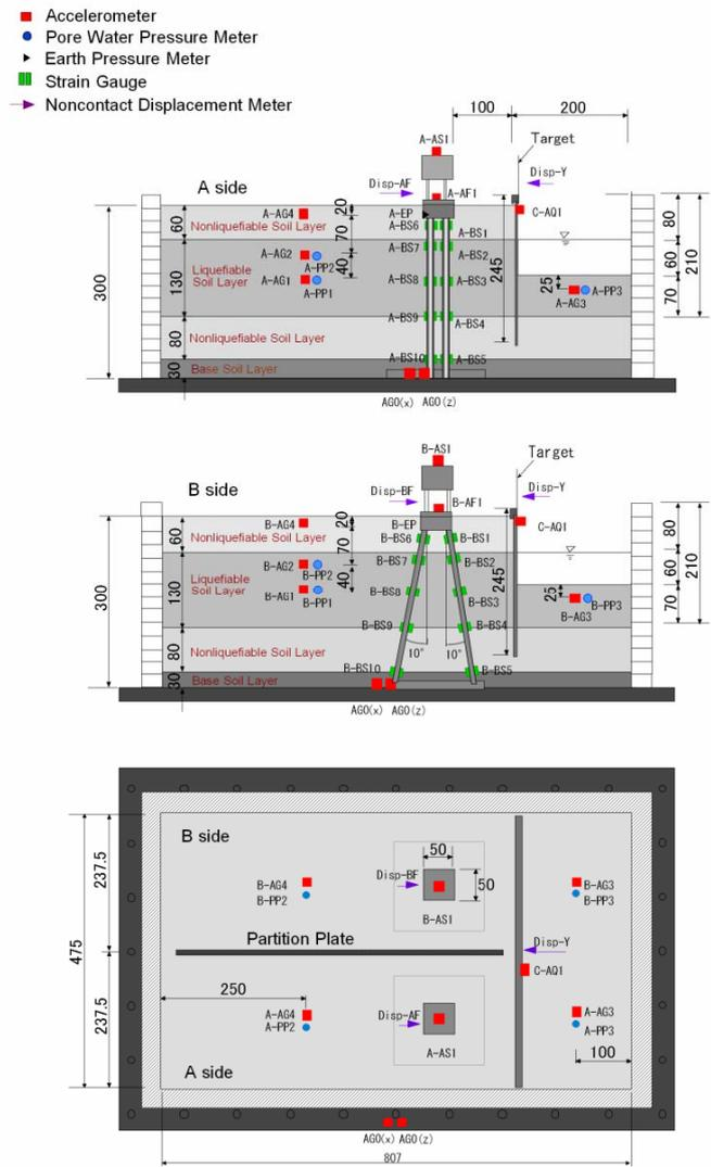
Figure 6. Longitudinal sections and plan of the 1/30-scale centrifuge model of Case 32 (scale unit: mm)
