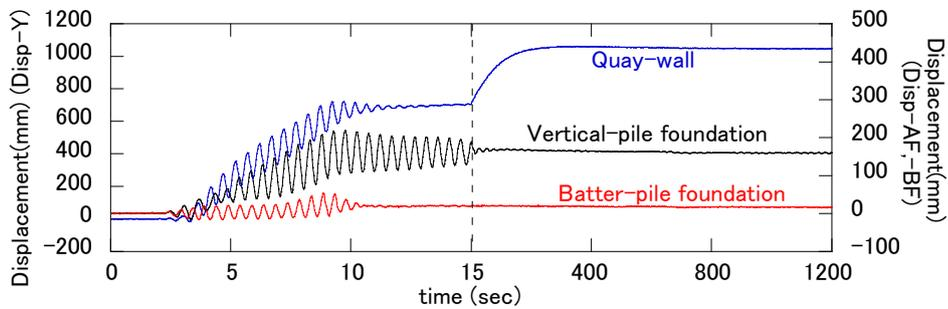
Figure 7. Time histories of the horizontal displacements of the quay-wall (Disp-Y), and the footings of the vertical piles in A-side (Disp-AF) and of batter piles in B-side (Disp-BF)
