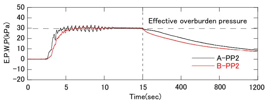
Figure 2. Excess pore water pressure records in the second soil layer (Case 2)
