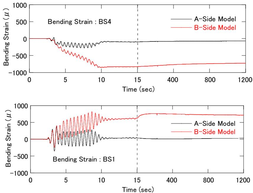
Figure 5. Comparison between the bending strains of the pile-heads and pile-tips at A-side and B-side (Case 2)
