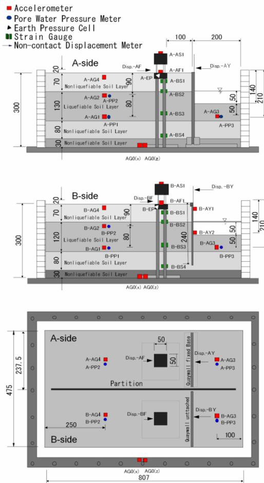
Figure 1. Longitudinal sections and plan of the 1/30-scale centrifuge model of Case 2 (scale unit: mm, for the prototype dimensions: multiply by 30)
