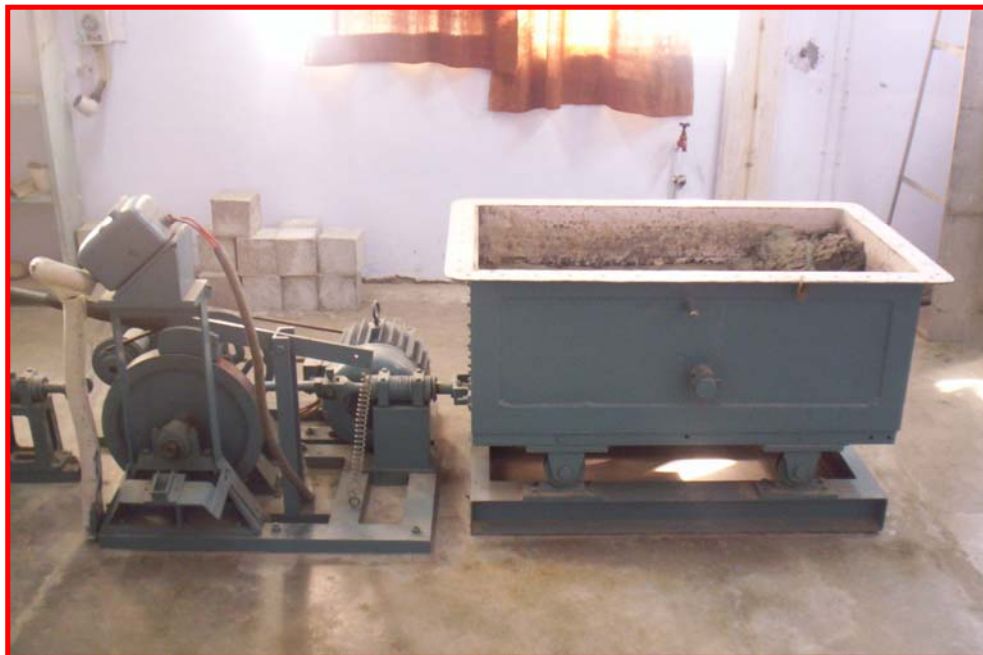
Fig. 1: Liquefaction Table at Dept. of Earthquake Engineering, IIT Roorkee
