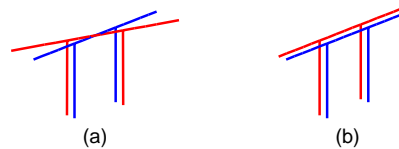
Figure 6. Deflected shapes associated with the “effective” influence vector of a three-span symmetric bridge: (a) excitation in fault-parallel direction; and (b) spatially-uniform excitation.
