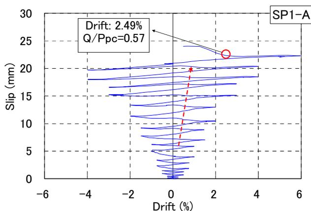
Figure 3.6 Beam slip vs. story drift, SP1-A
