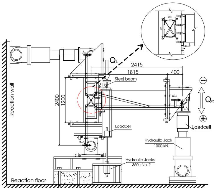
Figure 2.2 Test set up
