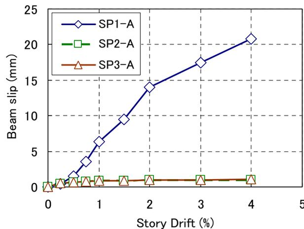
Figure 3.5 Beam slip-story drift relationship of all specimens
