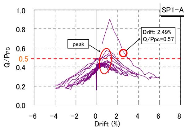
Figure 3.7 Beam shear force/ PC force, SP1-A
