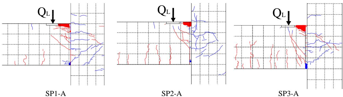
Figure 3.1 Crack patterns of the specimens after 4% drift
