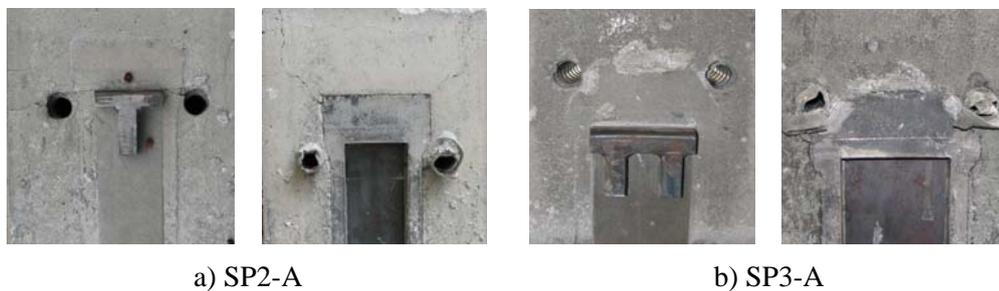
Figure 3.2 Shear bracket and U-shaped steel box after the test
