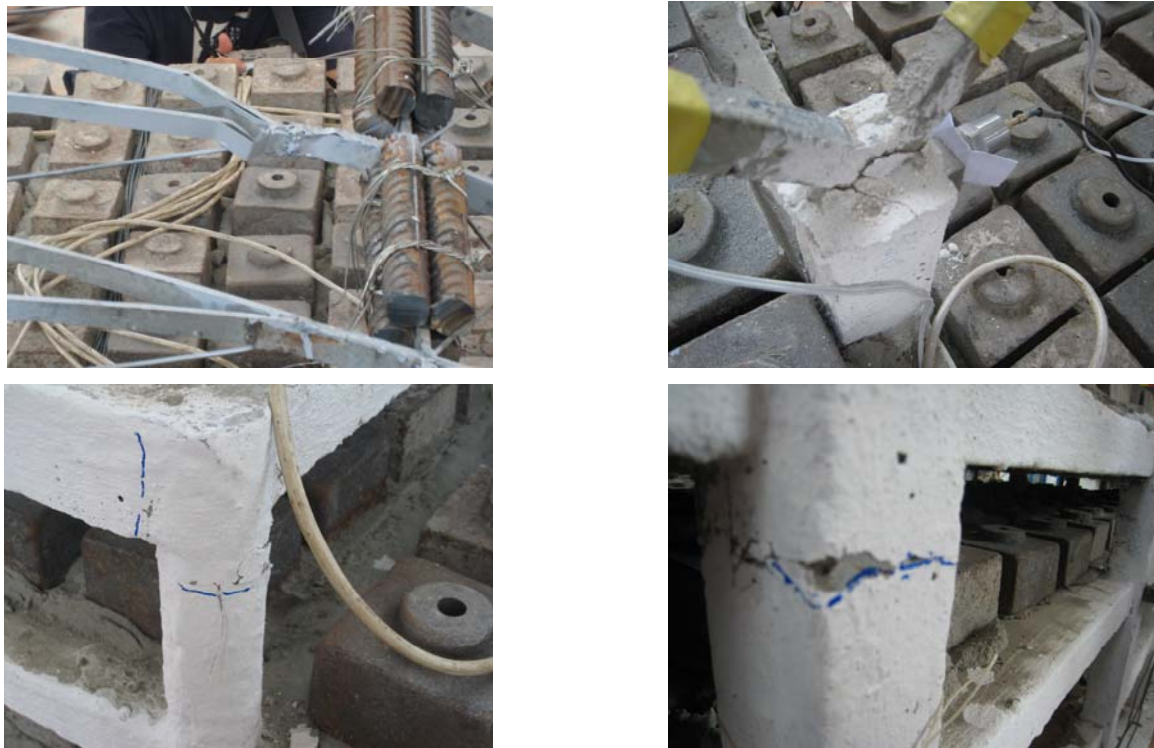
Figure 4 Failure pattern of test model
