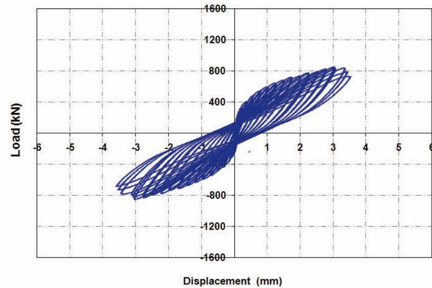
Figure 5 Hysteretic loops of SW3 model under cyclic loading
