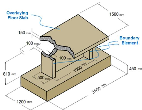
Figure 1 laboratory tested shear wall with boundary elements
