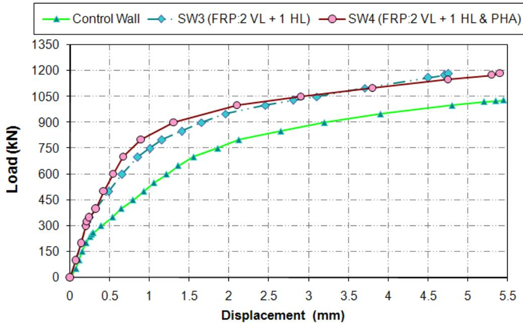
Figure 4 Comparison of load-displacement curves for “Control wall”, “SW3” and “SW4”.
