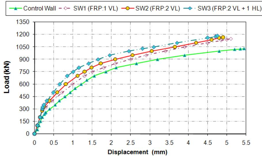
Figure 3 FE analysis load-displacement curves for structural models
