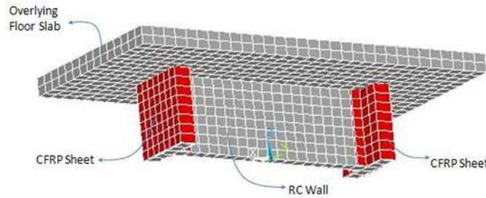
Figure 2 Finite Element model of RC walls externally bonded with FRP sheets.
