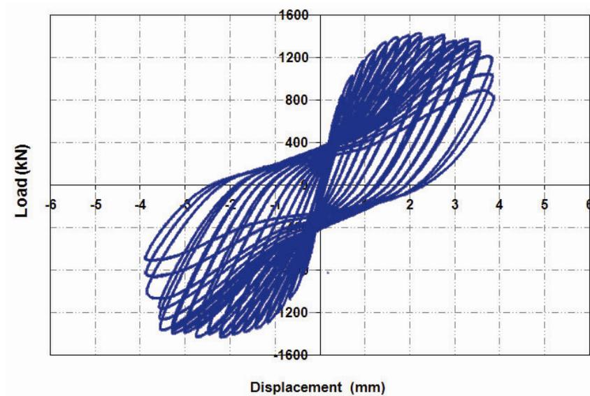
Figure 6 Hysteretic loops of SW4 model under cyclic loading
