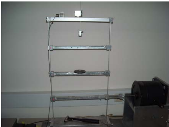
Figure 8 Three-storey frame with TMD
