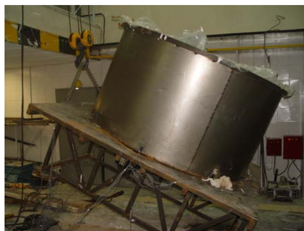
Figure 4 Experimental investigation of broad tank model
