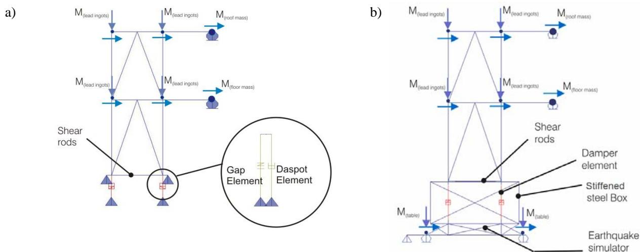
Figure 4 Numerical models used for the analysis of the VDCSR system:
