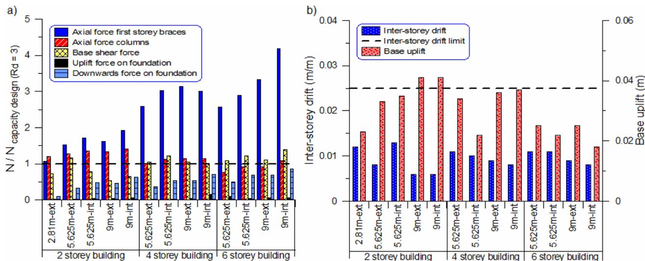
Figure 2 Mean peak response parameters of the VDCSR system applied to 2-, 4- and 6-storey buildings located in Montreal: a) Force demand in the VDCSR system relative to current code capacity design forces; b) Displacement response with the VDCSR system.
