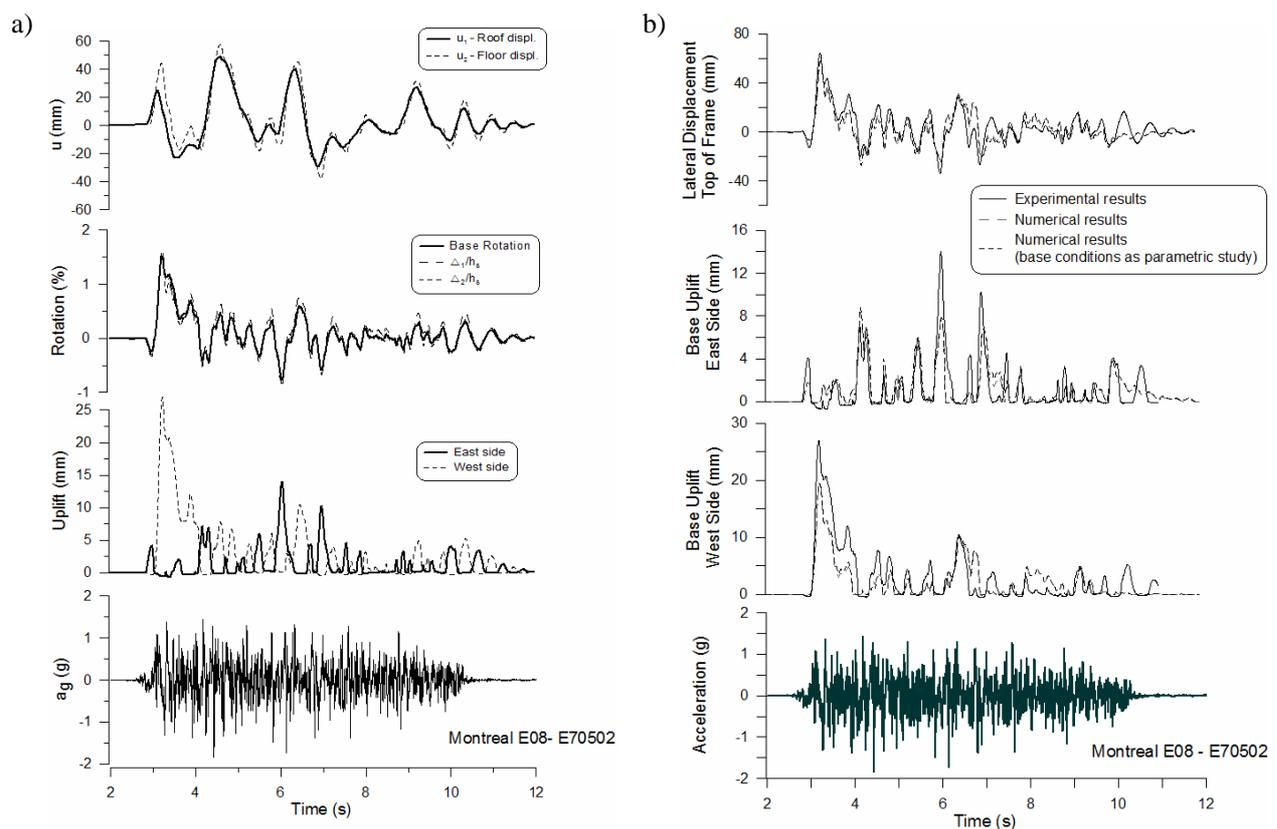
Figure 7 Shake table test under an M7.0 at 50 km seismic event for the Montreal site:
