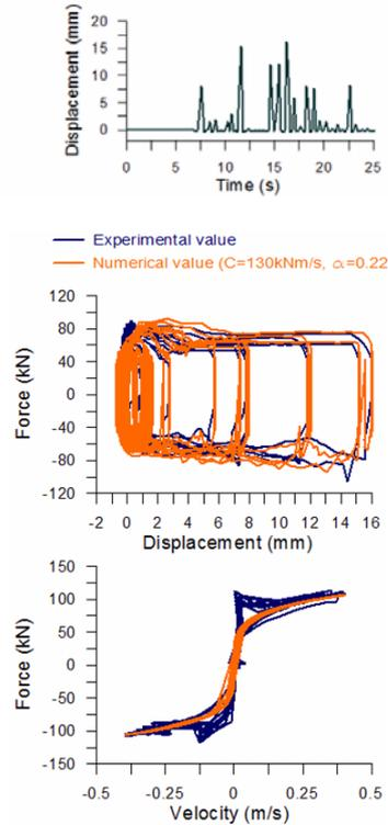
Figure 5 Characterization of the damper units under: a) Harmonic sinusoidal signal; b) Uplift time histories of the model structure under an M7.0 at 50 km seismic event for Montreal.
