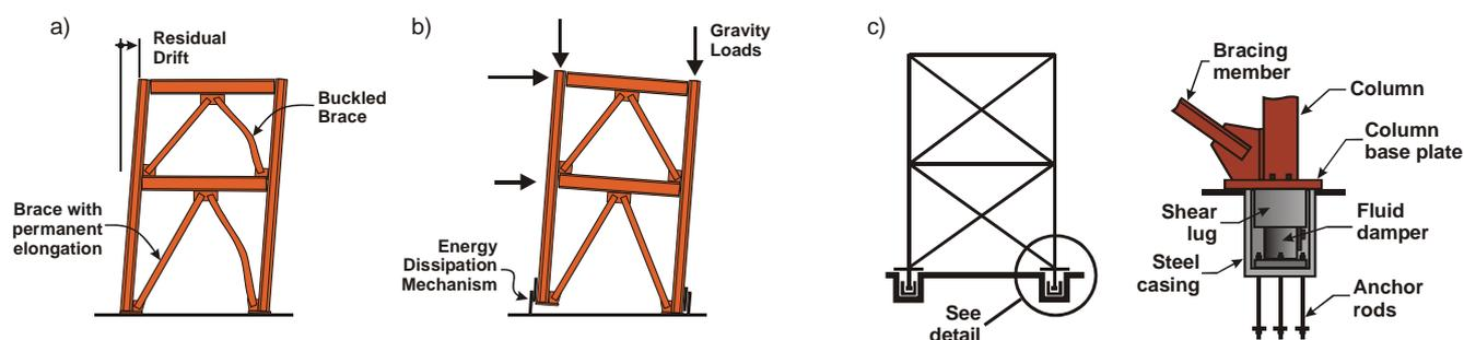
Figure 1 a) Expected seismic damage in concentrically braced steel frames; b) Rocking braced frame; and c) Proposed viscously damped controlled seismic rocking (VDCSR) braced steel frame system.
