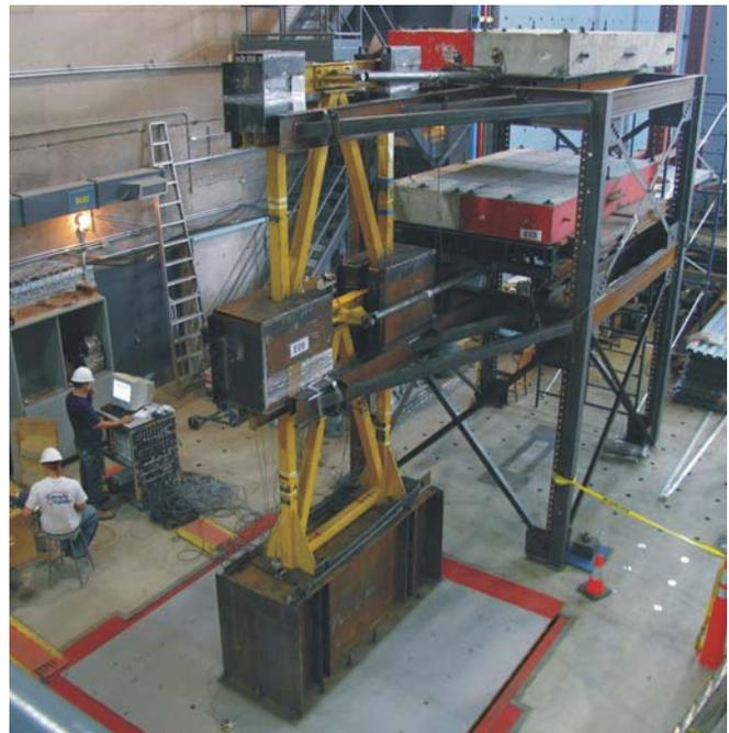
Figure 6. Shake table test setup: a) Schematic of the test model; b) Entire test setup with seismic mass system.
