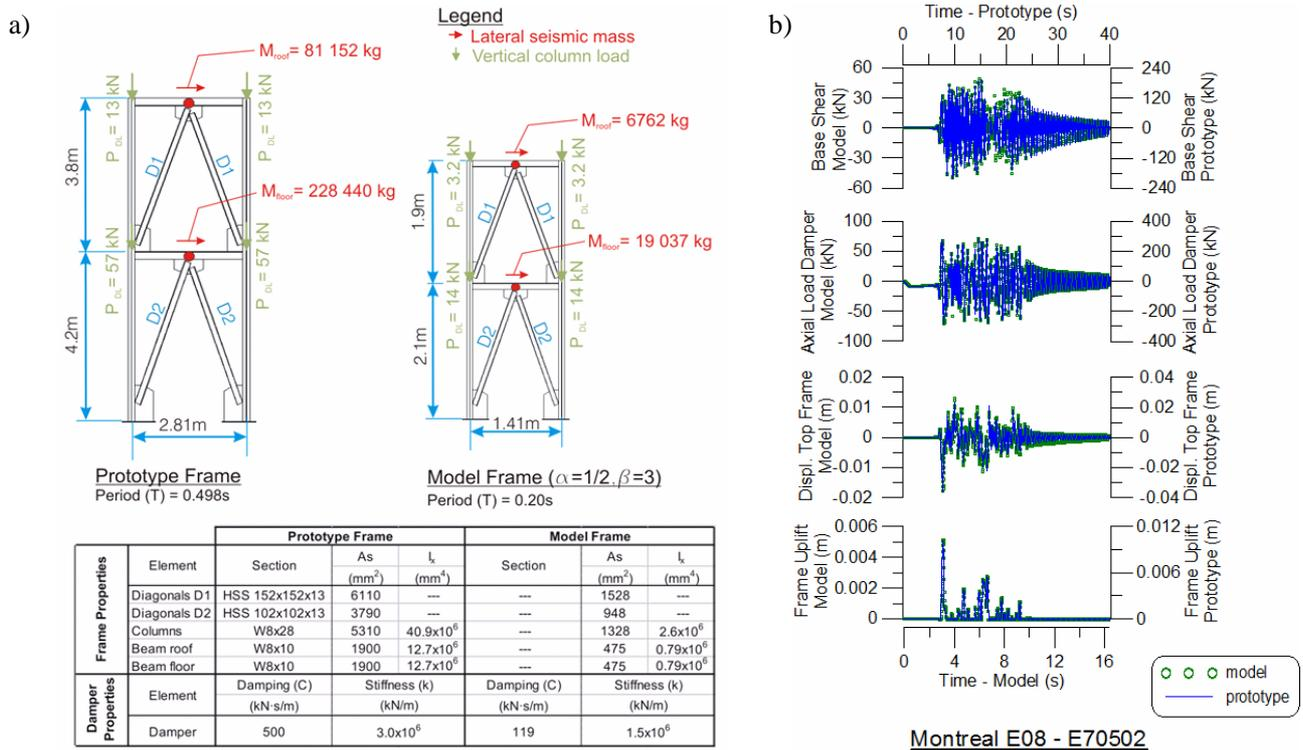
Figure 3 Design and validation of the test model: a) Characteristics of the prototype and model structures; b) Comparison of the response of the prototype and model to an M7.0 at 50 km seismic event for Montreal.
