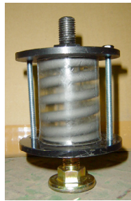
Fig.4 Damper with coil spring used for the test
