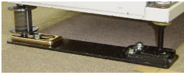
Fig.3 Overturn prevention device for lightweight structure
