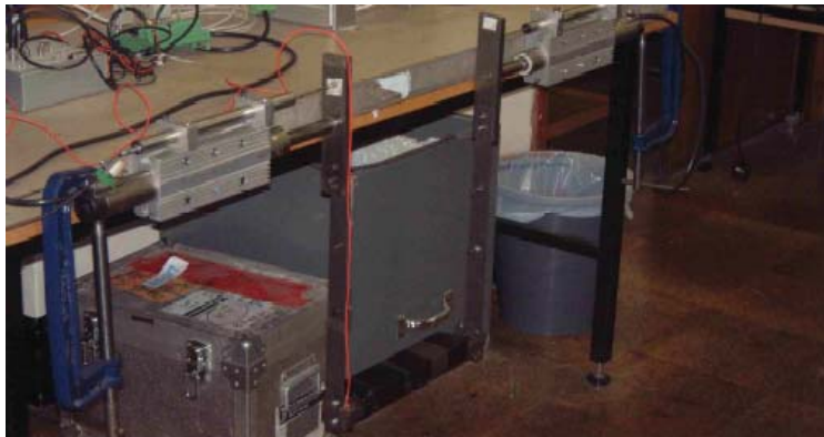
Figure 1. The single (inverted) portal frame MSE experimental set up.
