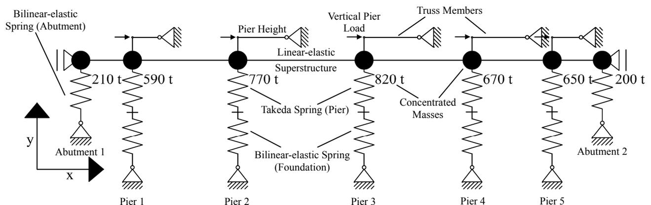
Figure 7 Dynamic system of bridge structure for inelastic dynamic analysis (in plan view)
