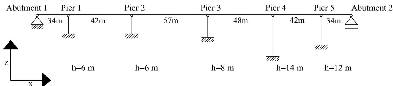
Figure 1 Bridge structural system
