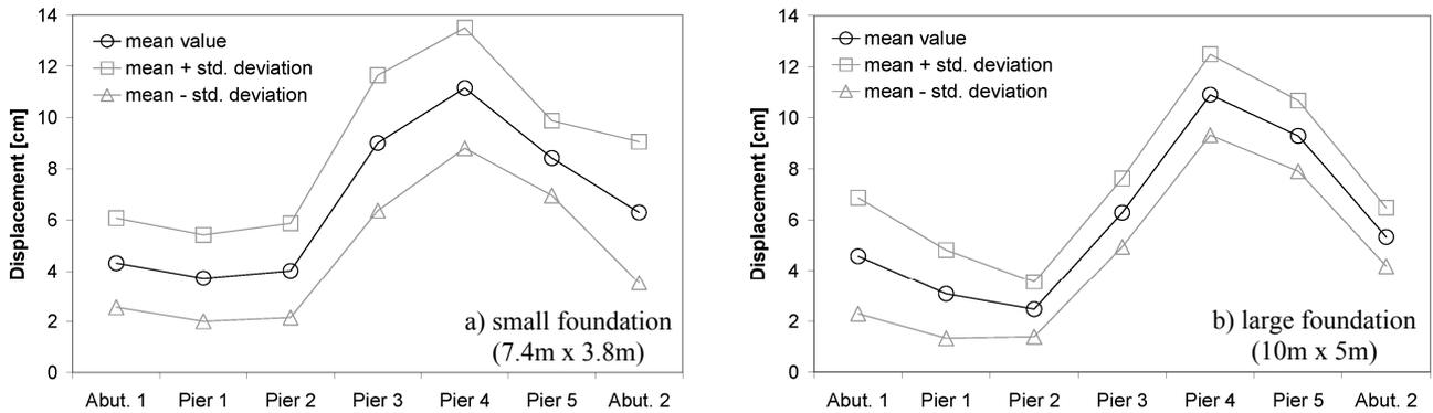
Figure 9 Peak total displacements for piers with spread-foundations
