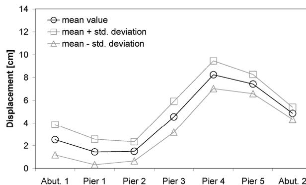
Figure 8 Peak total displacements for rigidly fixed pier bases
