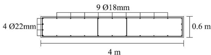
Figure 2 Cross-section of piers
