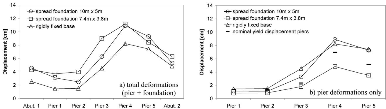
Figure 10 Comparison of peak displacements for structures with different foundation types
