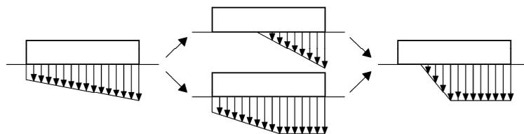
Figure 5 Soil pressure under spread foundations from moment and vertical load
