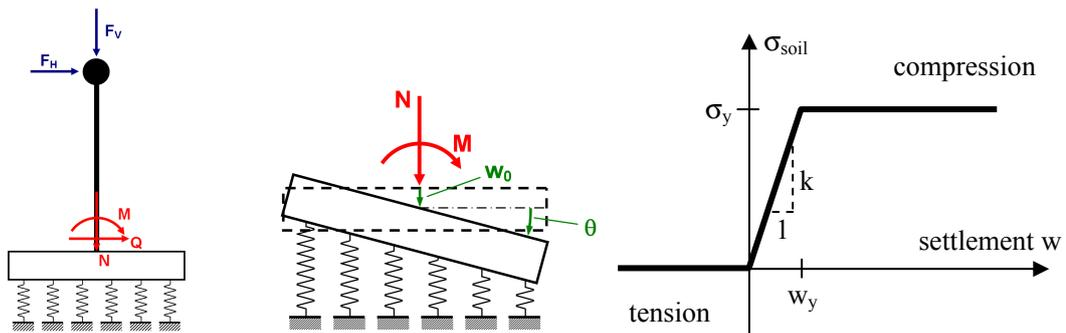
Figure 4 Soil-foundation model with bilinear-elastic Winkler springs
