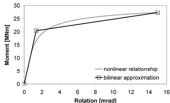
Figure 6 Moment-rotation relationship of a 10m x 5m spread foundation
