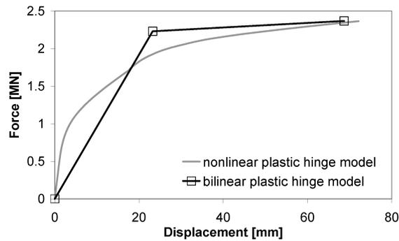
Figure 3 Force-displacement relationship of a 8 m pier
