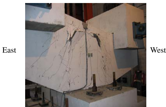
Figure 7 Damage in the irregular beam
