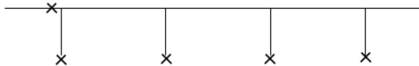
Figure 15 The flexural crack initiated at the first span and bottom of all piers at PGA = 0.27g
