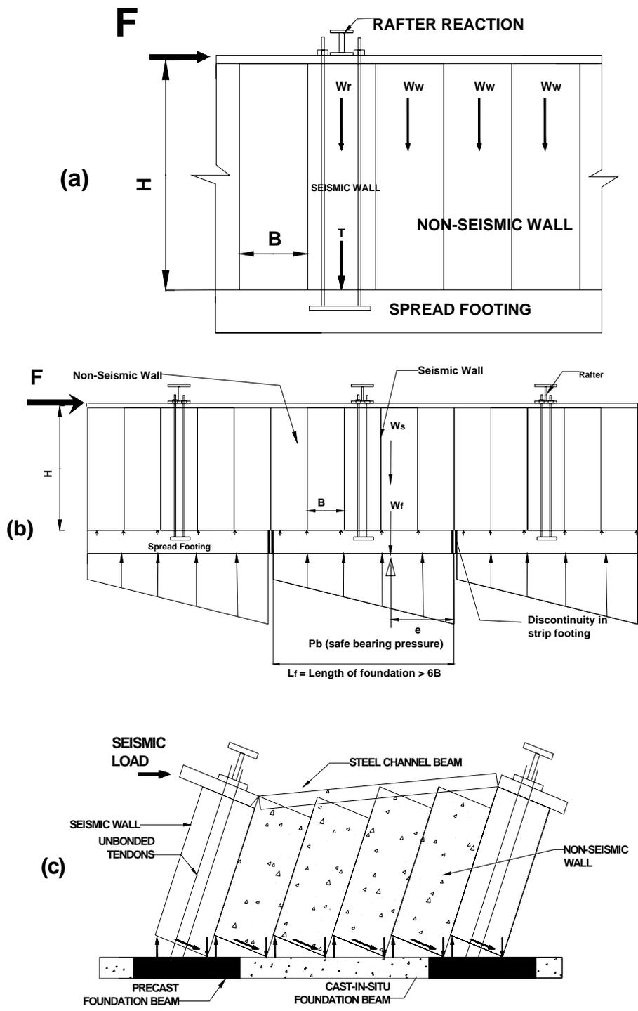
Figure 2: The forces and interaction of multi-panel acting on spread footing; (a) seismic resistance in multi-panel wall system; (b) distribution of soil bearing pressure underneath spread footing; and (c) interaction between multi-panel walls and spread footing during ground shaking.
