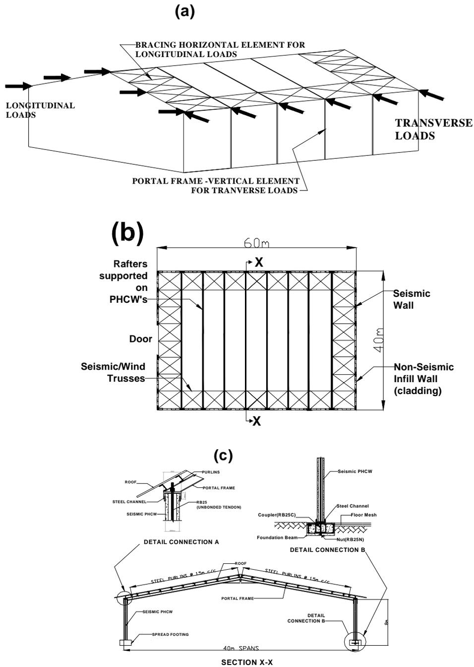
Figure 1: Concept overview of warehouse building; (a) distribution of transverse and longitudinal loading arising from either wind or earthquake effects; (b) plan view of warehouse showing lines of portal frames seated on PHCW; and (c) steel portal frame setting on PHCW together with detailing connection at top and bottom of the wall.
