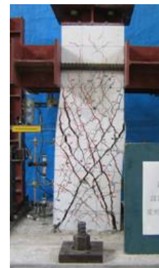
Figure 4.3 Crack patterns at the final stage
