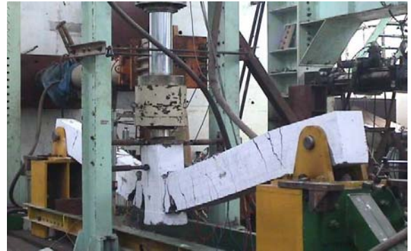
(a) Collapse ultimate state
