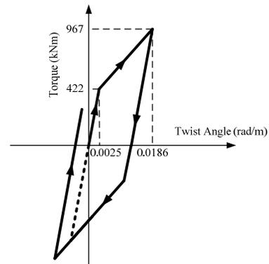
Figure 3.5 Bilinear Hysteretic Torque-Twist Relationship of Wall
