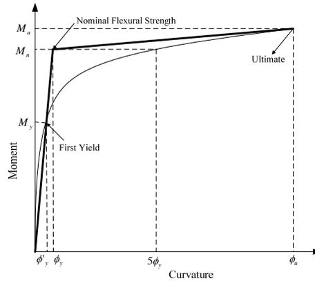
Figure 3.2 Idealization of Bilinear Moment-Curvature Relationship
