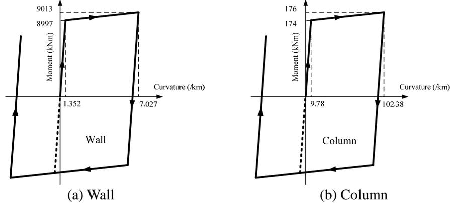
Figure 3.3 Bilinear Hysteretic Moment-Curvature Relationship of Wall and Column
