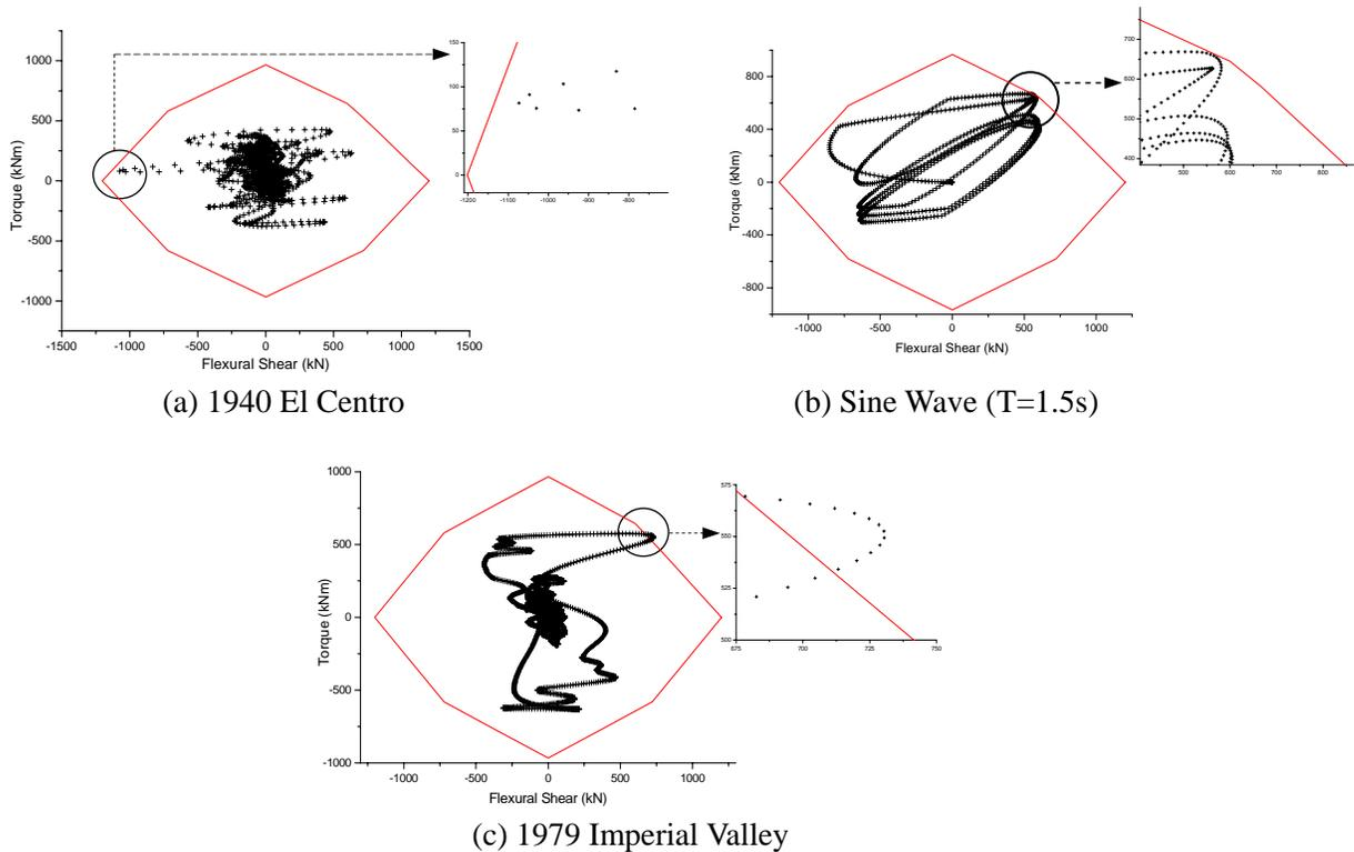
Figure 3.6 Shear and Torque Histories of Wall of Reference Model A
