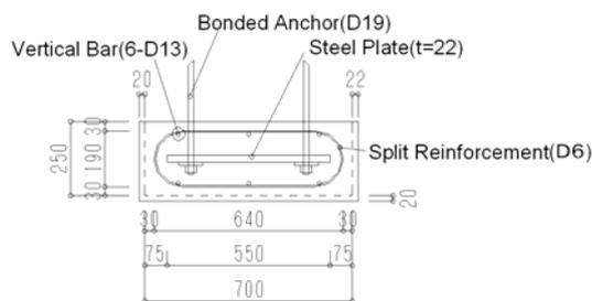
Fig.4.5 Existing-Additional Column Connection
