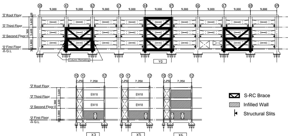
Fig.4.1 Arrangement of Retrofitting Members in Elevation and Sections
