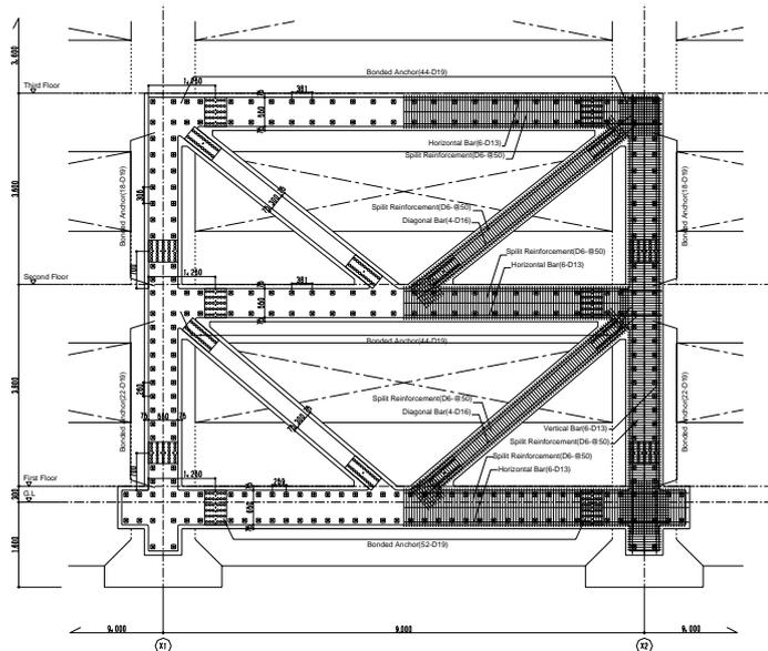
Fig.4.3 Details of R/C Brace with a Built-In Steel Plate (S-RC Brace)
