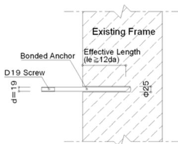
Fig.4.4 Embedded Length of Bonded Anchor Used in S-RC Brace
