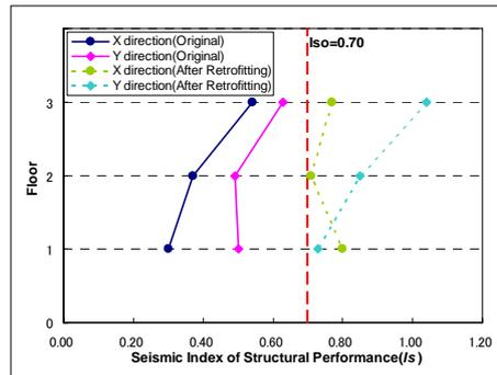
Fig.5.2 Comparison Between Before and After Retrofitting  $I_s$ -Index
