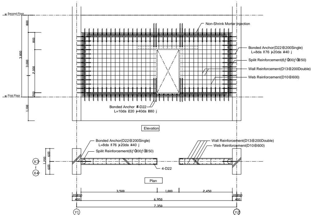
Fig.4.6 Details of Retrofitting RC Shear Wall with Opening
