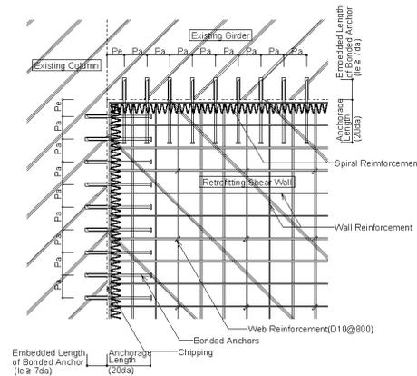
Fig.4.7 Detail of Retrofitting Shear Wall
