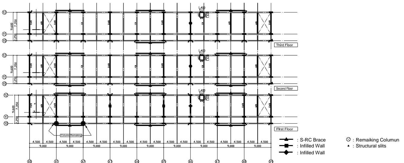
Fig.4.2 Arrangement of Retrofitting Members in Plans of Each Floor
