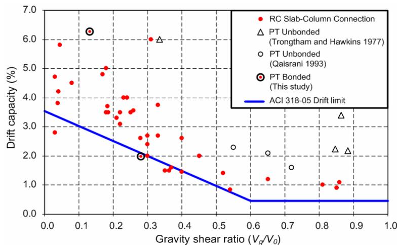
Figure 6 Gravity shear ratio versus drift capacity at punching for RC and PT slab-column connections
