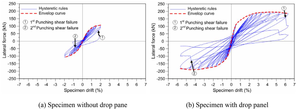
Figure 5 Lateral force-drift results of both specimens
