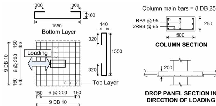
Figure 4 Bonded reinforcing bars in drop panel and column of the specimen with drop panel
