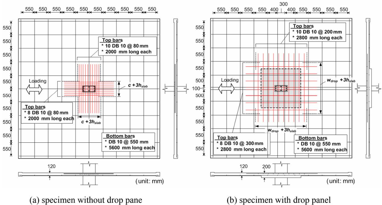
Figure 3 Bonded reinforcing bars in slabs
