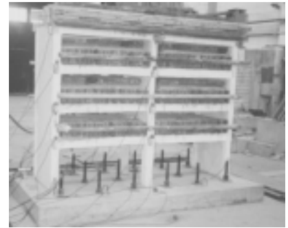
Figure 1 Model fixed on shaking table
