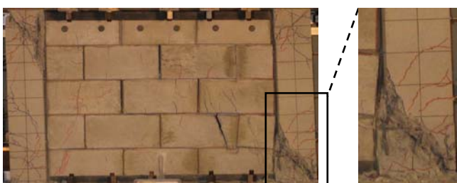
Photo 2 Damage to I-Frame (R) after in-plane loading
