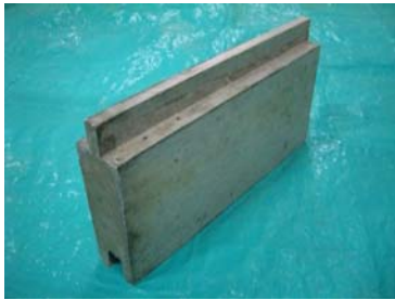
Figure 1 Prototype of interlocking block capable of resisting out-of-plane loads
