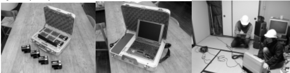
Figure 2 Portable Vibration Measurement Machine, Velocity-meters and Measuring Microtremor Scene
