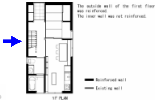
Fig.12 Retrofit for Narrow House
