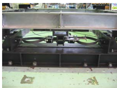
Figure 5 Lead damper installed in test specimen
