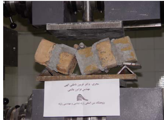
b: Flexural Tension Test
