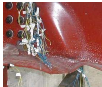
Fig 5 Flexure failure on the compressive flange of changed section
