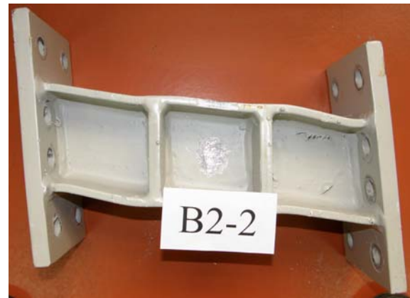
Figure 9. Specimen B2-2 of seismic link after testing
