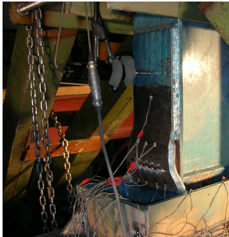
Figure 12. net section yield of the upper cover plate (SPC3)
