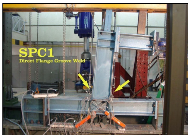
Figure3. Specimen 1 at final hysteretic displacement amplitude
