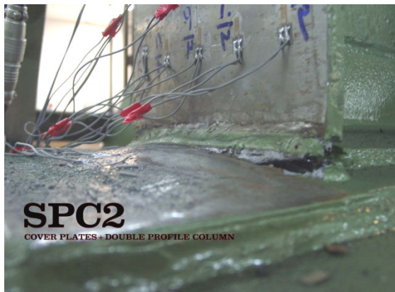
Figure8. Specimen 2- Buckling of the end plate and Crack propagation from the weld root
