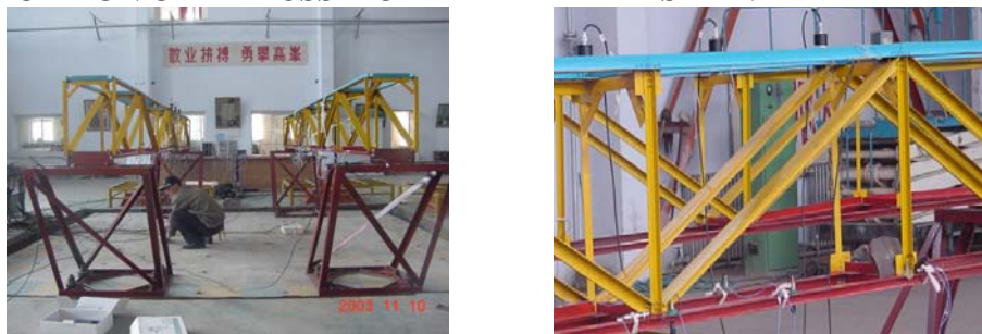
Figure 10 truss model arranged on shake-table (Left) and sensors placed on the test model (Right)
