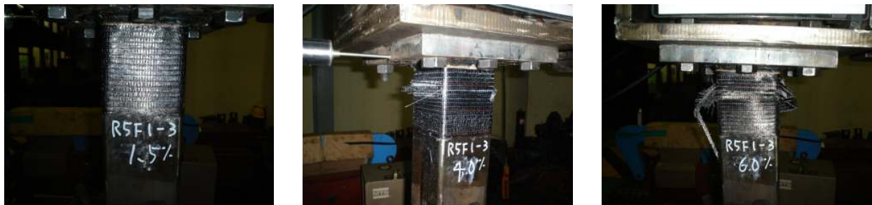
Figure 2 Failure procedure for TR-CFT column (R5F-3)
