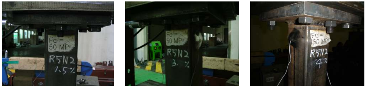
Figure 1 Failure procedure for conventional CFT column (R5N)
