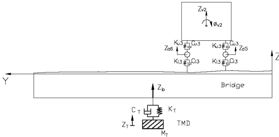
**Fig 1B: Dynamic Interaction Analytical Model Of The Vehicle-Bridge System - Sectional View.**
