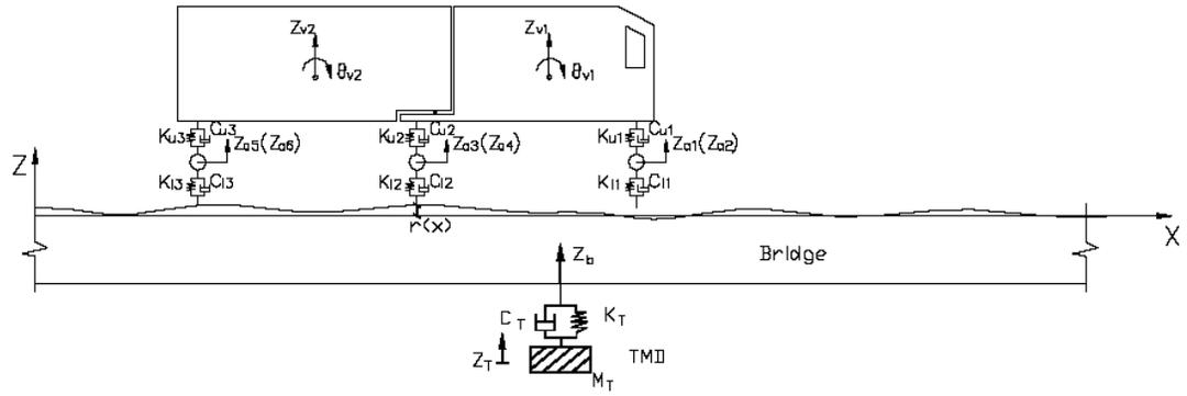
**Fig 1A: Dynamic Interaction Analytical Model Of The Vehicle-Bridge System - Longitudinal View.**
