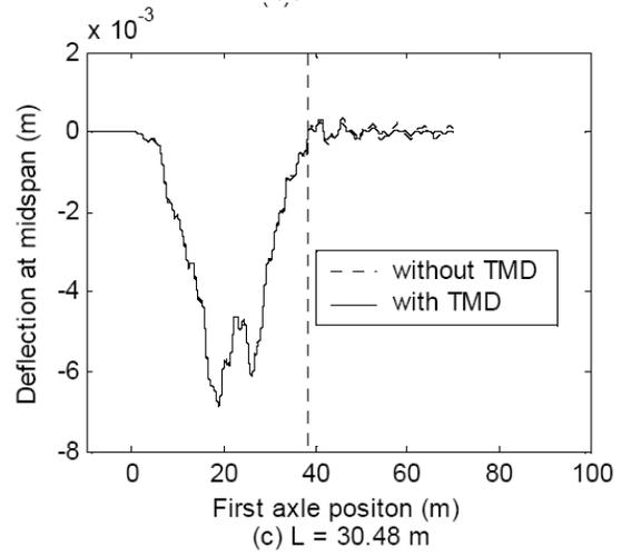
**Fig. 2: Time History Of Deflection At Mid-Span Of Slab Bridges With And Without TMD**
