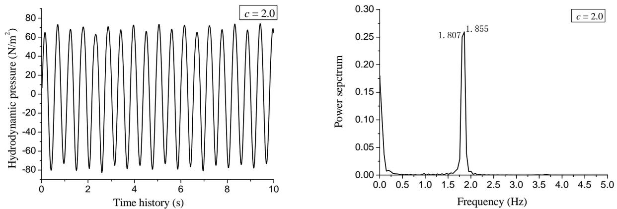
Fig8 Hydrodynamic pressure and corresponding power spectrum with varying exciting wave frequency ratio
