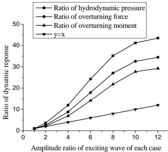
Fig6 Various dynamic responses ratio with varying amplitudes ratio of exciting wave
