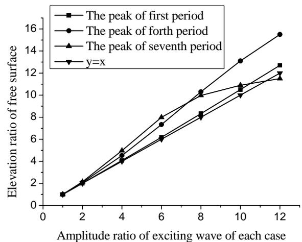
Fig5 Various elevation ratio of free surface at right side of the wall with varying amplitudes of ratio of exciting wave
