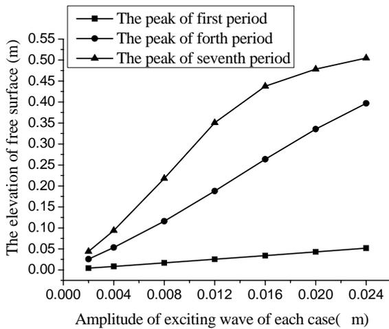
Fig4 Various elevation of free surface at right side of the wall with varying amplitudes of exciting wave
