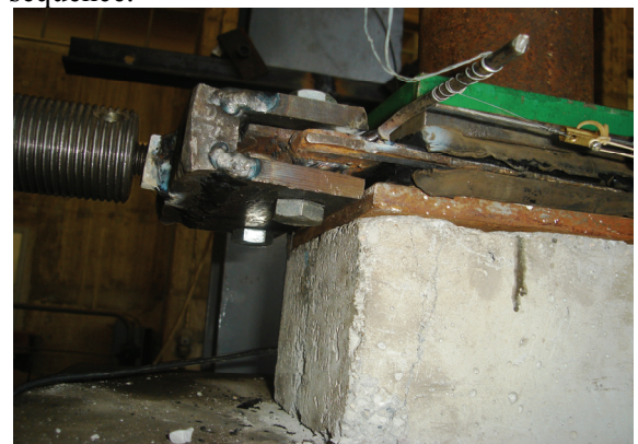
Figure 15. Failing mode of the unit slice specimen without the presence of the compressive stress field.
