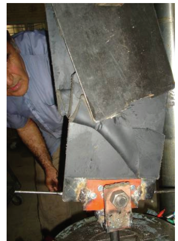
Figure 11b. Failing mode of the unit slice specimen without the presence of the compressive stress field.
