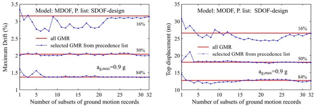
Figure 7. The 16%, 50% and 84% fractile of the maximum drift and top displacement as a function of the selected subsets of ground motion records for an  $a_{g,max}=0.9$  g and the precedence list of ground motion records defined from the results of the SDOF-design model.
