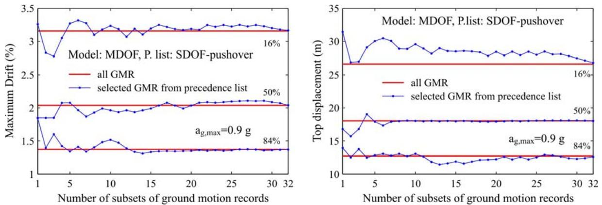
Figure 8. The 16%, 50% and 84% fractile of the maximum drift and top displacement presented as a function of the selected subsets of ground motion records for an  $a_{g,max}=0.9$  g and the precedence list of ground motion records defined from the results of the SDOF-pushover model.
