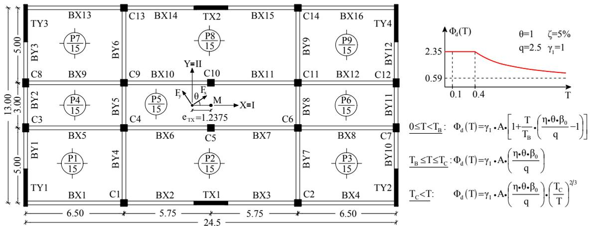
Figure 3 Plan view of a 5-storey symmetrical building (5SST<sub>xL</sub>) with  $T_x > T_C$  and  $T_B < T_y < T_C$
