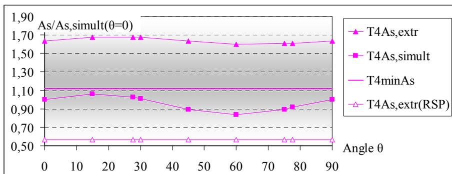
Figure 8 Longitudinal reinforcement for wall T4 of model 5SUNT<sub>L</sub> normalized with regard to the reinforcement derived using the probable simultaneous values of the sectional forces for excitation angle  $\theta=0^\circ$  with regard to principal axis I
