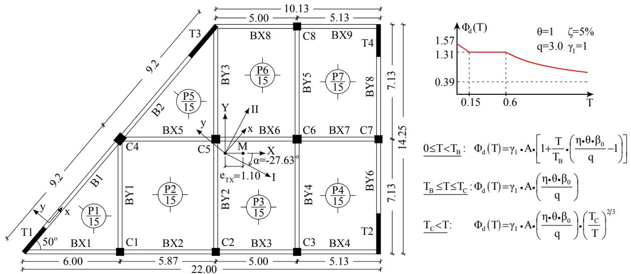
Figure 4 Plan view of a 5-storey non-symmetrical building (5SUNT<sub>L</sub>) with T<sub>i</sub> larger than T<sub>c</sub>
