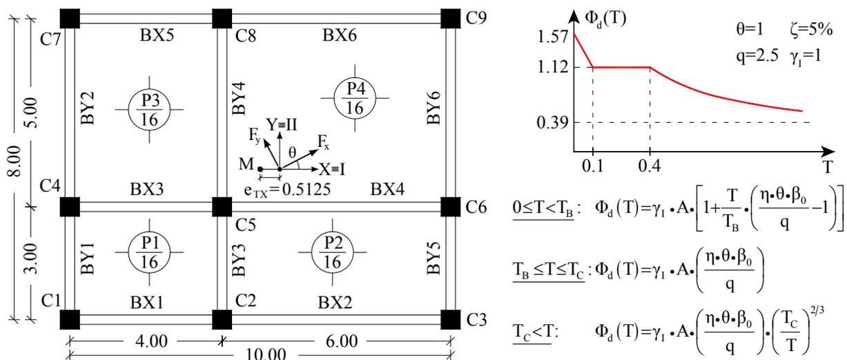
Figure 1 Plan view of a 3-storey unsymmetrical building (3SUNB) with  $T_i$  in the constant acceleration branch
