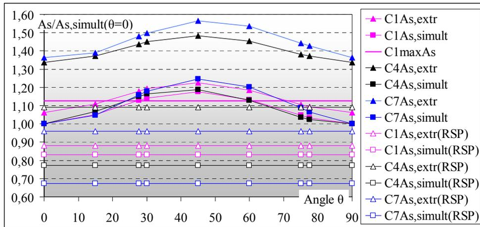
Figure 7 Longitudinal reinforcement for columns C1, C4 and C7 of model 5SUNT<sub>L</sub> normalized with regard to the reinforcement derived using the probable simultaneous values of the sectional forces for excitation angle  $\theta=0^\circ$  with regard to principal axis I
