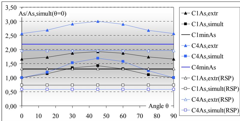
Figure 6 Longitudinal reinforcement of model 5SST<sub>xL</sub> normalized with regard to the reinforcement derived using the probable simultaneous values of the sectional forces for excitation angle  $\theta=0^\circ$
