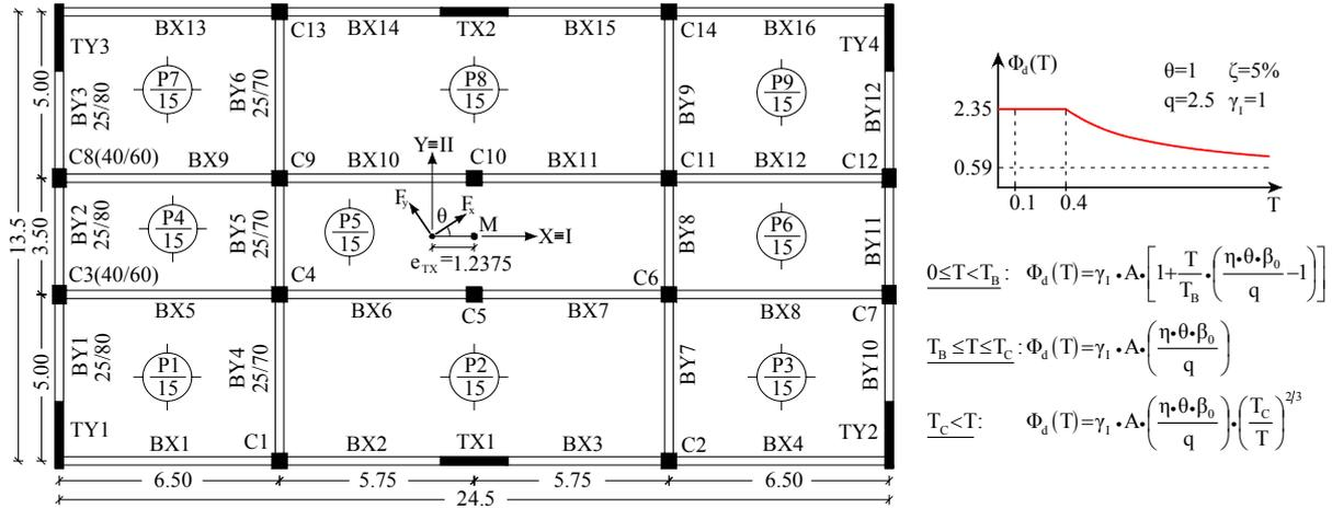
Figure 2 Plan view of a 5-storey symmetrical building (5SST<sub>L</sub>) with  $T_i > T_C$
