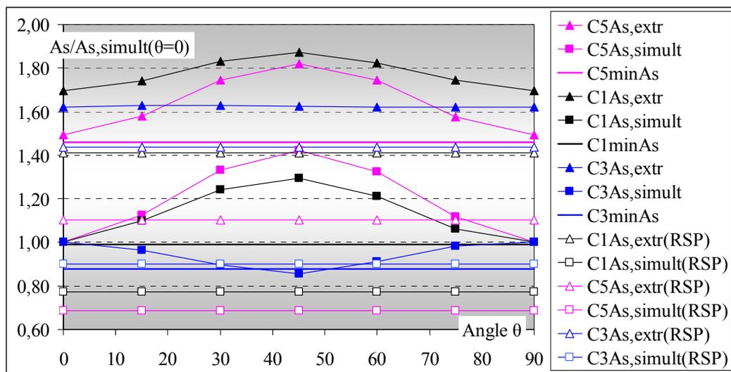
Figure 5 Longitudinal reinforcement of model 5SST<sub>L</sub> normalized with regard to the reinforcement derived using the probable simultaneous values of the sectional forces for excitation angle  $\theta=0^\circ$
