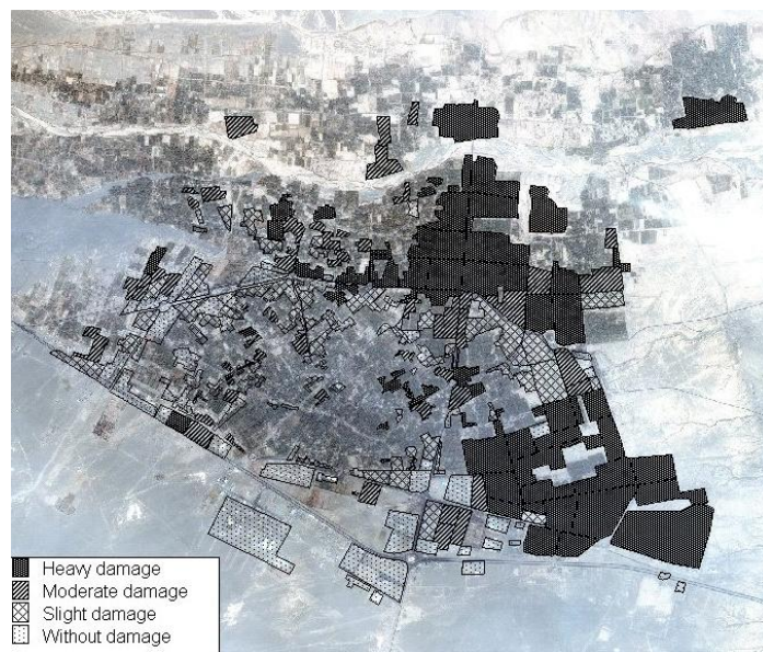
Figure 2 Estimation damages in Bam Earthquake (2003) using aerial photographs
