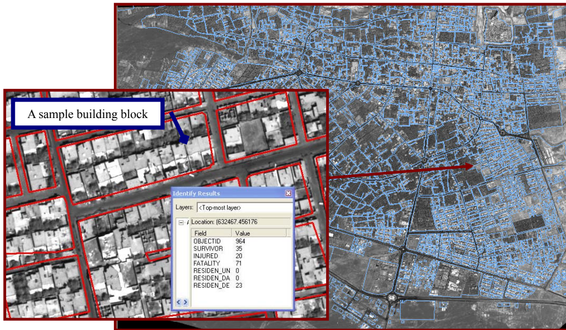
Figure 4 The BAM post disaster survey zones incorporated in GIS and overlaid on panchromatic optical image (includes: three levels of building damages in addition to three levels of human casualties)
