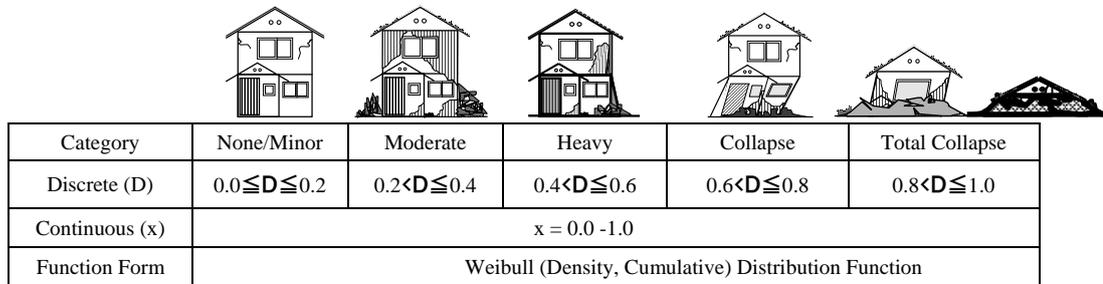
Figure 1 Classification of damage states of wooden dwelling houses with damage pattern chart.
