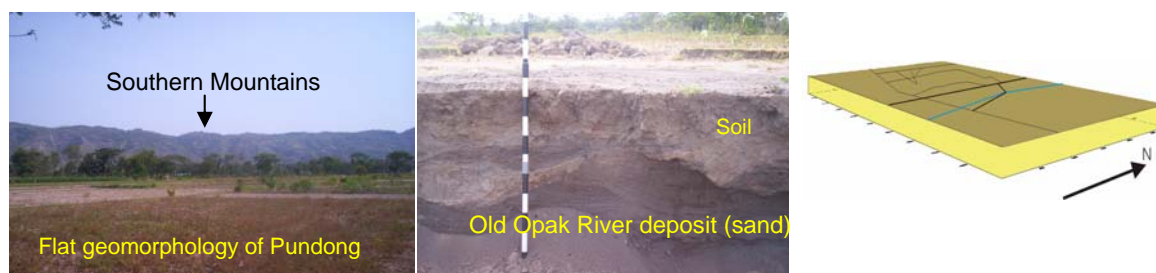
Figure 2. Illustration of flat morphology and thin soil above loose sand deposit in Panjangrejo Village, Pundong area.
