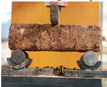
Fig. 4 Bending test device
