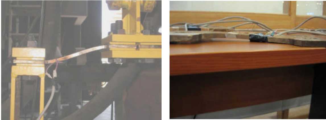
Figure 8, permanent deformation after 40 mm out of plane displacement
