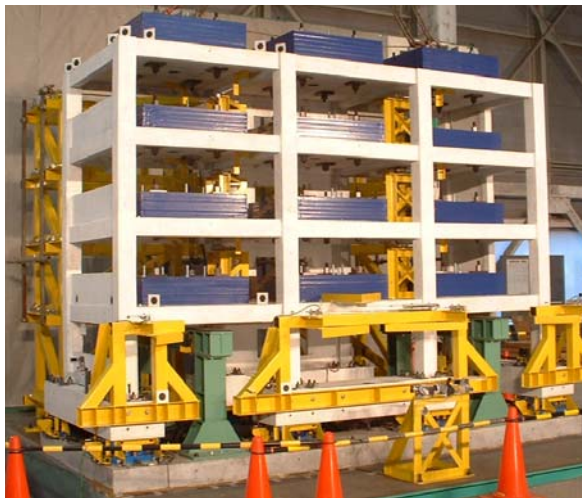
Picture 3 RC building model on the shaking table in dynamic experiment(left) and Smart AE sensor(right). The upper right figure shows the arrangement of SAE sensors.
