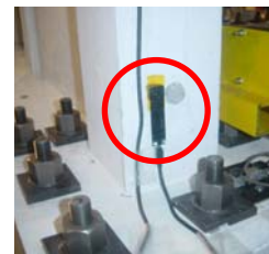
Picture 3 RC building model on the shaking table in dynamic experiment(left) and Smart AE sensor(right). The upper right figure shows the arrangement of SAE sensors.
