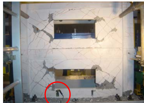
Picture 4 Cracked RC building model with sensor A at the foot of the column in the side of the waist wall(left) and sensor E at the foot of the opened wall(right).
