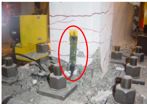
Picture 4 Cracked RC building model with sensor A at the foot of the column in the side of the waist wall(left) and sensor E at the foot of the opened wall(right).
