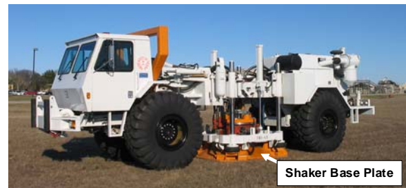
Figure 2 Tri-axial vibrator called T-Rex that is used as a high-energy, controllable-waveform, downhole source (from Stokoe et al, 2008)
