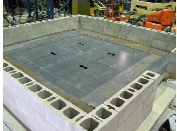
Figure 4 Setup of Isolated Floor System II
