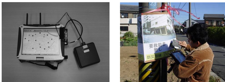
Photo 3 Intelligence sharing function with RFID tag. Left: System equipment. Right: Equipment in use.
