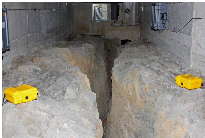
Figure 2 Sites IS608 and IS608b of the ICEARRAY network, serving a dual purpose. In this case an earthquake fault in the bedrock underneath the service center building in Hveragerdi, South Iceland, is monitored by two CUSP-3Clp units. One unit is a part of the ICEARRAY network and the other has the purpose of monitoring the differential motions across the fault during other earthquakes. The gray boxes on the base walls contain the auxiliary power and modems for the CUSPs.
