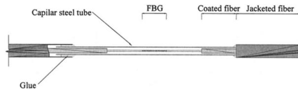
Figure 7. Scheme of the Temperature Sensor
