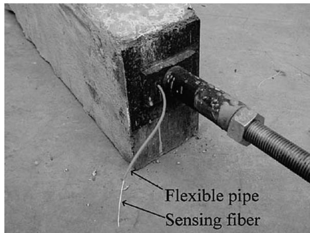
Figure 11. Photograph of a Beam Strengthened with FRP Cable
