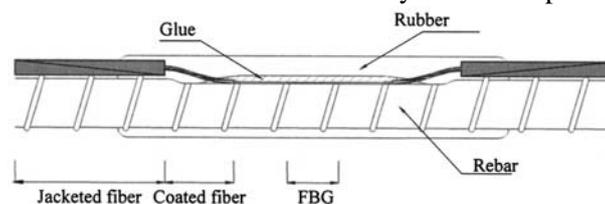
Figure 6. Scheme of the Strain Sensor
