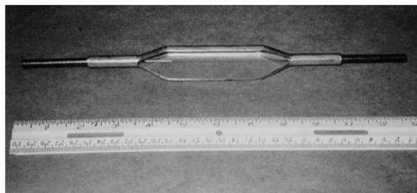
Figure 4. Photograph of a Stress Sensor
