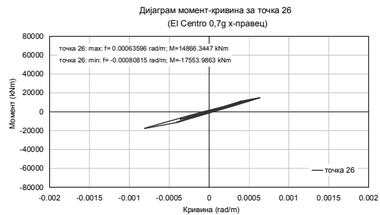
Fig. 19: El-Centro, 0.7g: Base Moment-Curvature Hysteretic Response of the Right Pier, x-direction: NP=26.
