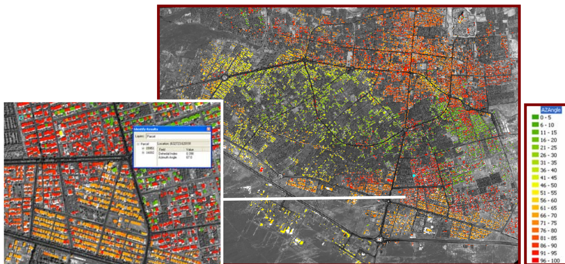
Figure 7 Simplified SAR for the most visible walls – Bam
